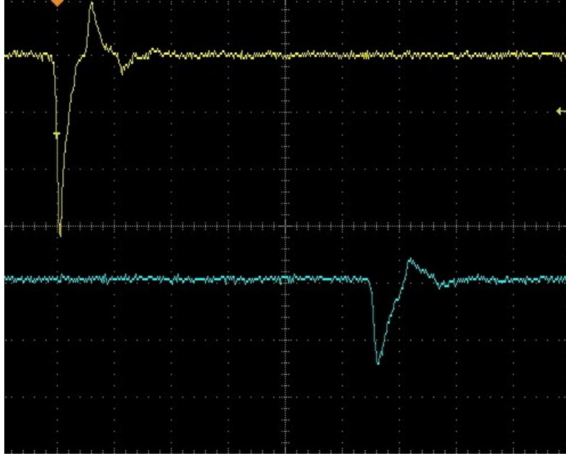
Fig.1a. Comparison of the pulse from an ultra-fast scintillation detector (yellow) and the same pulse after 200 ns standard delay (blue).
