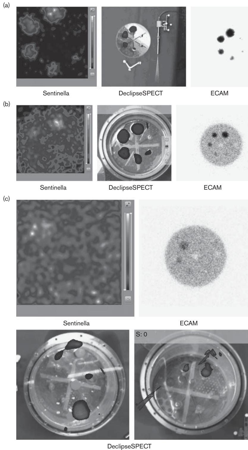
Comparison of scintigraphic images of the portable camera, freehand single-photon emission computed tomography (SPECT), and a conventional gamma camera. (a) Infinite contrast. (b) Contrast level of 1:8, spheres on surface of the background activity. (c) Comparison of scintigraphic images of the portable camera and the conventional camera at a contrast level of 1:8 with totally immersed spheres; the two images of the freehand SPECT show that reproducibility may be poor under this condition.
