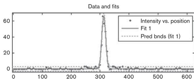
Measurement of full-width at half-maximum by curve fitting with MATLAB. Example of an ideal condition: conventional camera with a phantom volume of 5.5 ml at infinite contrast. Pred bnds, 95% confidence prediction bounds.
