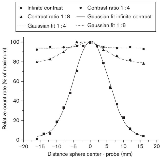
Count rates of the conventional probe for the 0.5 ml phantom sphere on the surface of the background activity.
