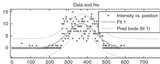
Example: conventional camera with a totally immersed 5.5 ml sphere at a contrast level of 1:8. Automatic calculation of full-width at half-maximum was not possible due to low image contrast. Pred bnds, 95% confidence prediction bounds.
